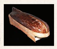
Step 6: Glue. Glue and epoxy are poured evenly into the inside of the hull. Top quality, wood glue is used adequately for planking and to make sure the hull will not split due to humidity changes.
